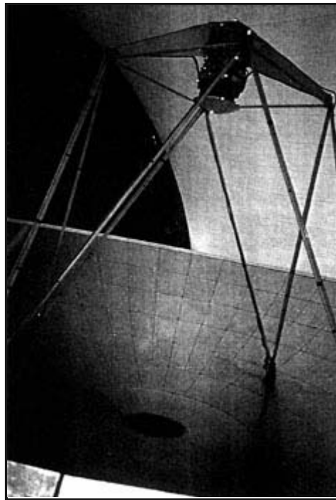
Figure 9. The primary 15-meter diameter surface of the JCMT on Mauna Kea, one of the few large facility designed to operate at Extreme InfraRed wavelengths. Also shown are the small secondary surface as supported by legs, and at right the windscreen.
