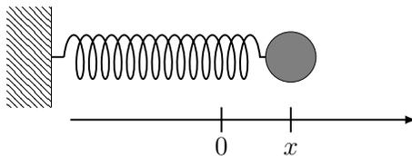
Figure 100: Harmonic oscillator: particle on a spring
