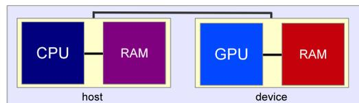
In so-called hybrid compute nodes (Fig. 36), one has one or several ordinary CPUs coupled to one or several GPUs, or other accelerator cards such as the new Intel Xeon Phi. Of course, these hybrid nodes can be clustered again with a fabric to form powerful supercomputers. In fact, the fastest machines in the world are presently of this type.
